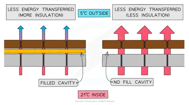
Less energy is transferred by conduction and convection if the cavity is insulated
